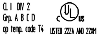
Figure 11: Printing on text detail in accordance with NEC
