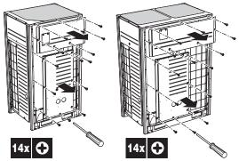
Once the front panel open, the electrical component box can be accessed by removing the control box cover as follows.
