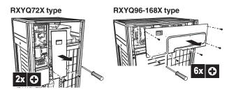
For service purposes, the push buttons on the main printed circuit board need to be accessed. To access these push buttons, the control box cover does not need to be opened. See 13. Making field settings on page 24.
