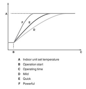
No matter which control is selected, variations on the behavior of the system are still possible due to protection controls to keep the unit operating under reliable conditions. The intentional target, however, is fixed and will be used to obtain the best balance between energy consumption and comfort, depending on the application type.
