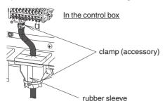
How to pass wire through the rubber sleeve:
