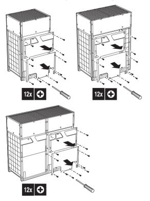
Once the front panel open, the control box can be accessed by removing the control box cover as follows.
