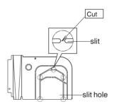
When side connections, remove the through hole cover on the bottom frame and lead out the piping from the bottom frame.
