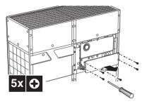
For service purposes, the push buttons on the main printed circuit board need to be accessed. To access these push buttons, the control box cover does not need to be opened. See 13. Making field settings on page 26.
