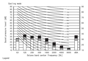
dBA = A-weighted sound pressure level (A scale according to IEC)
