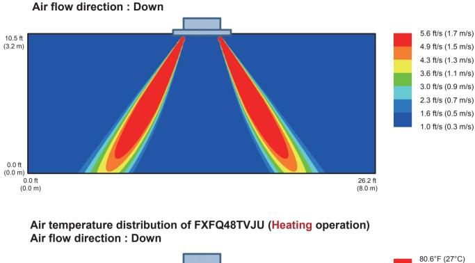
Air velocity distribution of FXFQ48TVJU (Heating operation)
