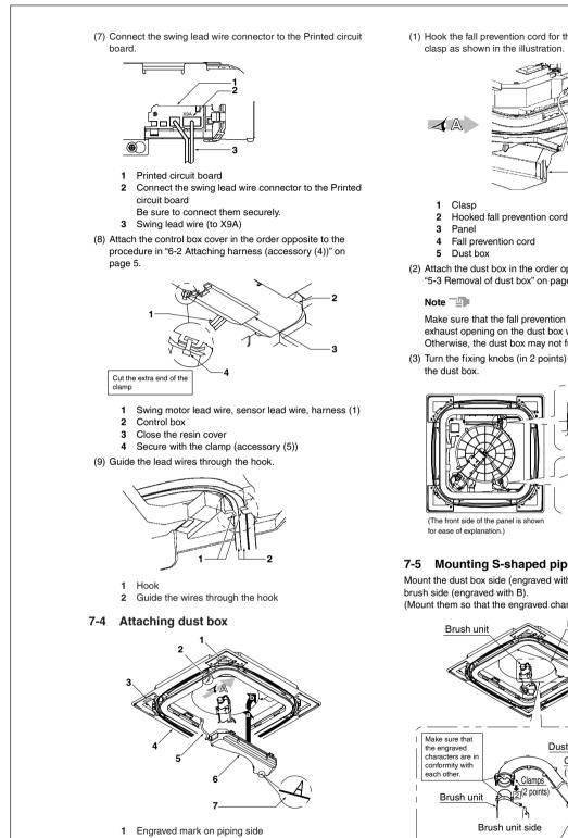
(1) Hook the fall prevention cord for the dust box to the panel clasp as shown in the illustration.
