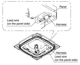
(3) Connect the connector of the lead wires and move the glass tube to cover the connector part.
