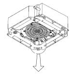
(1) Remove the bypass hole closing cap.
