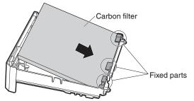
2 While pushing the hooks up, set the carbon filter under the 2 hooks.
