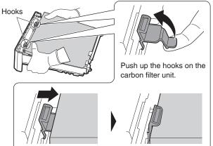
Securely attach the filter with the hooks.
