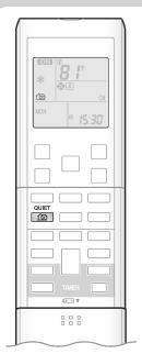
OUTDOOR UNIT QUIET operation lowers the noise level of the outdoor unit by changing the frequency and fan speed on the outdoor unit. This function is convenient during the night.
