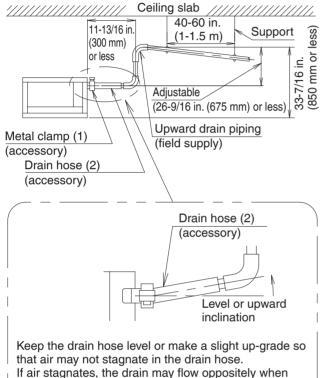
the drain pump stops and generate abnormal sound.
