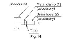
Do not tighten the metal clamp (1) with the torque more than the specified value. The drain hose (2), the socket or the metal clamp (1) may be damaged. • Wrap the vinyl tape around the end of the metal clamp (1) so that the sealing material (Large) (6) to be used at the next process may not be damaged with the clamp end or bend the tip of the metal clamp (1) inward as shown. (Refer to Fig. 15)
