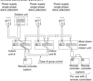
Note) There is not need to set the indoor unit address when using group control. (It is automatically set when the power is turned on.)
