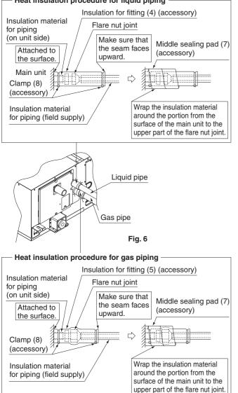
Use the insulation for fitting (4) and (5) provided to the liquid piping and gas piping, respectively, and conduct heat insulation work.
