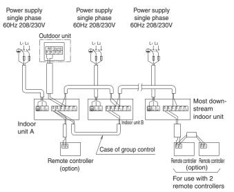
Note) There is not need to set the indoor unit address when using group control. (It is automatically set when the power is turned on.)
