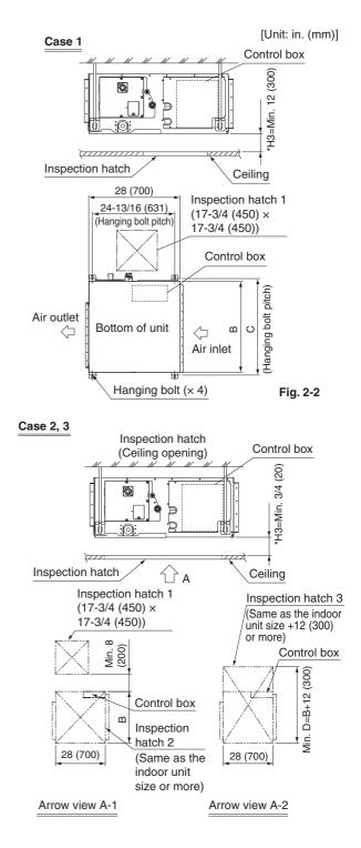
• Determine the H3 dimension by maintaining a downward slope of at least 1/100 as specified in 7. DRAIN PIPING WORK.
