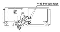
• After all the wiring connections are done, fill in any gaps in the through holes with putty or insulation (procured locally) to prevent small animals and insects from entering the unit from outside. (If any do get in, they could cause short circuits in the control box.)
