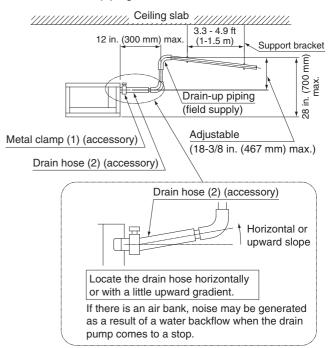
(2) Check the smooth draining of the piping on completion of the installation of the piping.
