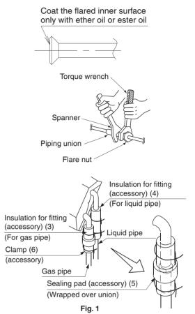
Use "Table 3" as a reference if a torque wrench is not available. Once work is complete, make sure there is no gas leaking. As the flare nut is tightened with the wrench, the torque will suddenly increase. From that position, tighten the nut to the angle shown on "Table 3".
