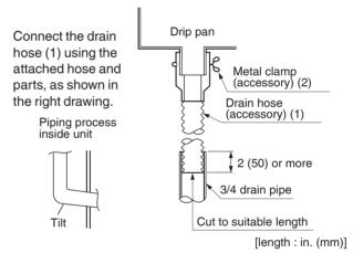
• If converging multiple drain pipes, install according to the procedure shown below.
