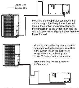
Insulation is necessary to prevent condensation from forming and dropping from the suction line. Armflex (or satisfactory equivalent) with 3/6" min. wall thickness is recommended. In severe conditions (hot, high humidity areas) 1/2" insulation may be required. Insulation must be installed in a manner which protects tubing from damage and contamination.
