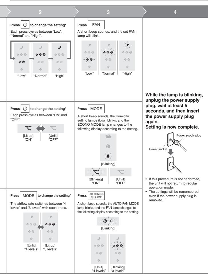
\* If the lamps do not change even after the settings were changed, unplug the unit, wait at least 5 seconds, then re-insert the power supply plug and repeat the above procedure from the beginning.
