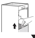
② Hold the bottom of the dust collection filter and pull it out.
