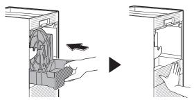
If the humidifying filter unit is not properly attached to the humidifying tray, the humidifying tray cannot be attached to the unit.
