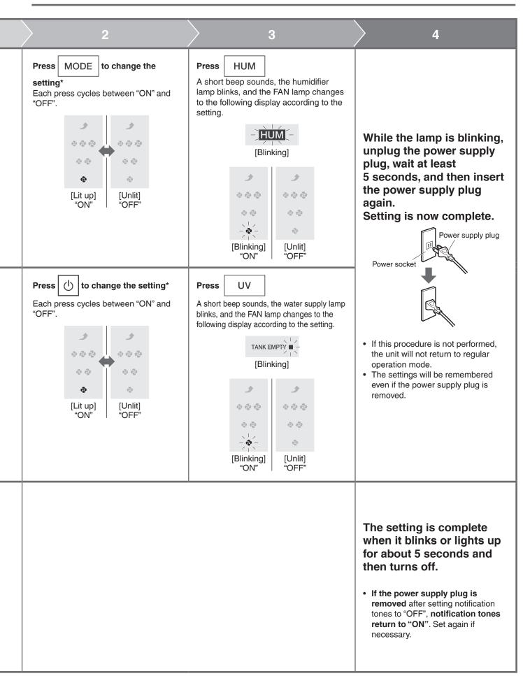
\* If the lamps do not change even after the settings were changed, unplug the unit, wait at least 5 seconds, then re-insert the power supply plug and repeat the above procedure from the beginning.
