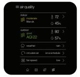
The air quality screen\* displays indoor air quality levels when a Daikin *One* home air monitor is connected. Outdoor air quality and weather will be displayed when the thermostat is connected to the internet and added to the mobile app.
