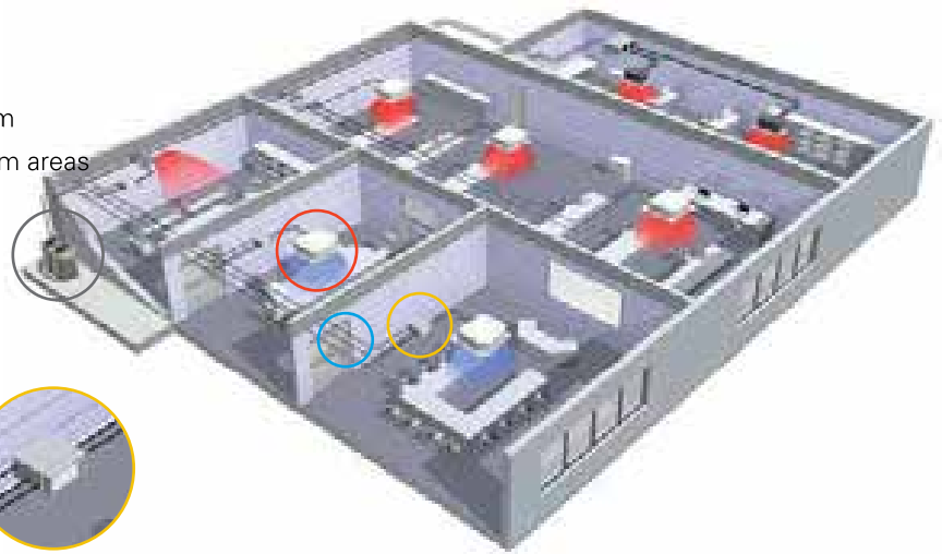
Single and multi Branch Selector boxes: allows the individual switching of indoor units between heating and cooling
