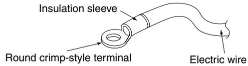
Connect wires of the same gauge to both sides.
