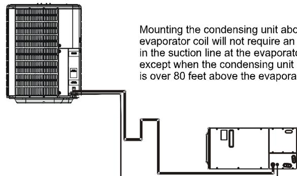
Insulation is necessary to prevent condensation from forming and dripping from the suction line. Armflex® (or satisfactory equivalent) with 3/8" min. wall thickness is recommended. In severe conditions (hot, high humidity areas) 1/2" insulation may be required. Insulation must be installed in a manner which protects tubing from damage and contamination.
