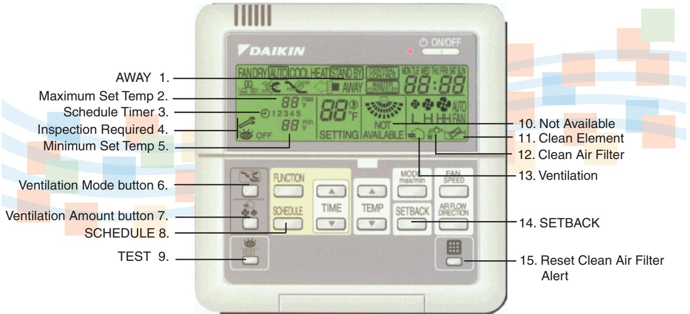
1. **AWAY:** The AWAY function prevents the room temperature from dropping or rising when the occupants are out for a period of time. If the room temperature drops below 50°F, heating is started automatically. As soon as 59°F is reached, the controller returns to its original status. If the room temperature rises above 85°F, cooling is started automatically. As soon as 74°F is reached, the controller returns to its original status. ON is enabled, flashing indicates ACTIVE, if disabled it is OFF.
